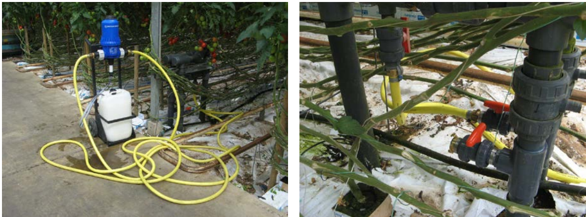
Figure 1. Dosatron in position for treatment (image left) and showing attachments to manifold (image right)
